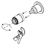
**01** Unscrew the handle with the help of the allen key.
