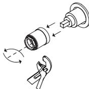
**04** Unscrew the tecaform locknut with the help of a wrench. After this, you can remove the cartridge.
